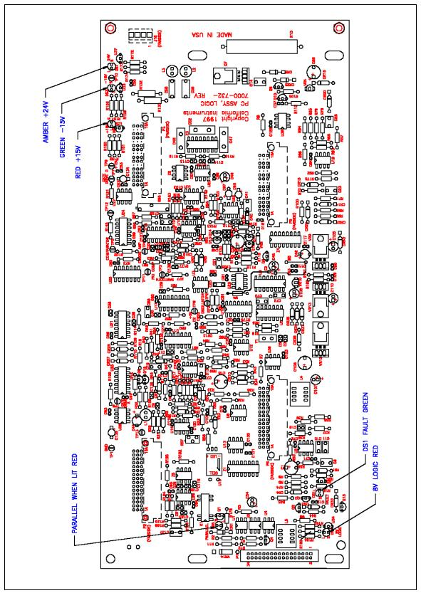
Figure 5-4: Logic Board LED's
