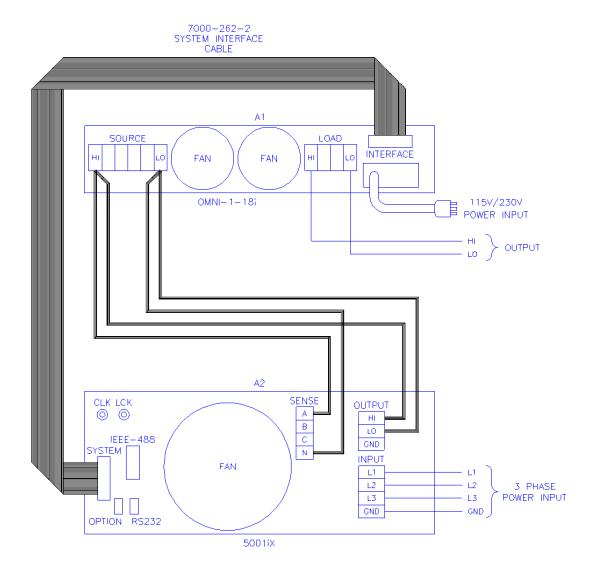
Figure 9-42: Example Connections With OMNI 1-18i
