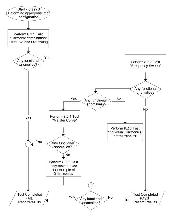
Figure 9-33: IEC 61000-4-13 Test Flowchart Class 3
