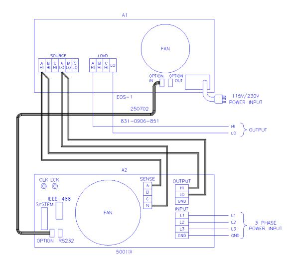
Figure 9-36: Example Connection With 5001iX and EOS-1
