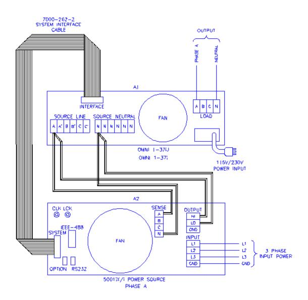
Figure 9-44: Schematic Showing OMNI 1-37i and 1-37iJ Connected to 5001iX System
