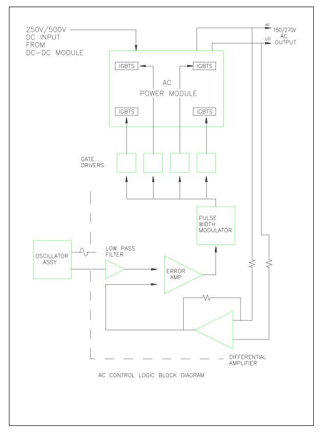
Figure 5-6: AC Control Logic Block Diagram
