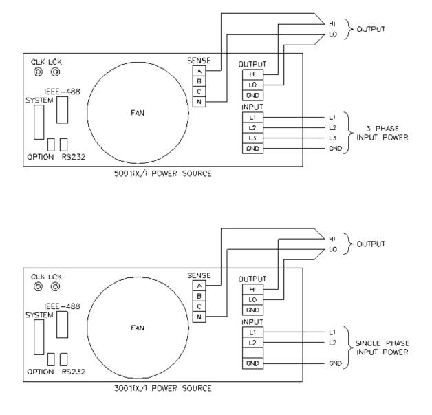
Figure 3-7: Connection For Single Power Source (5001iX/i, 3001iX/i)
