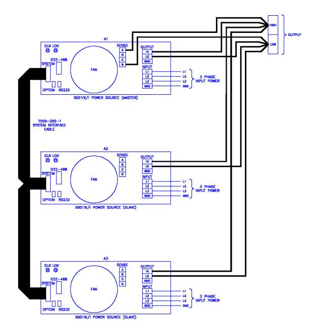
Figure 3-11: Single Phase 15000 VA System (15001iX/i)
