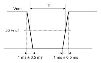
Switching Transients conform Figure B. The T1, T2 and T3 values are shown on screen in the table above the graph. Each permutation shown is repeated one time with a 1 second delay (default) between transients.
