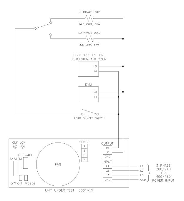
Figure 3-8: Functional Test Setup
