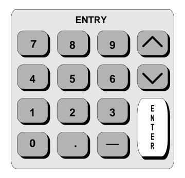
Figure 4-3: Entering value from decimal keypad
