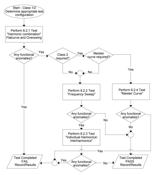
Figure 9-32: IEC 61000-4-13 Test Flowchart Class 1 and 2
