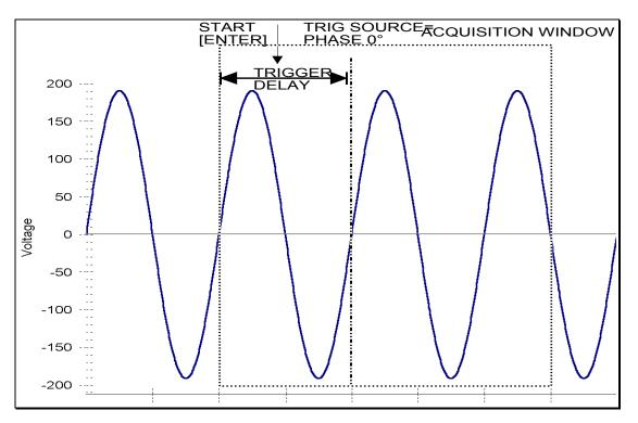
Figure 4-38: Negative trigger delay (Pre-trigger data)
