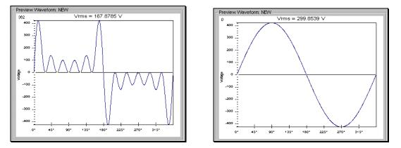
Figure 4-31: Waveform crest factor affects max. rms voltage
