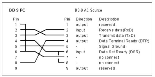
Figure 3-2: RS232C Cable for PC Connection wiring diagram.
