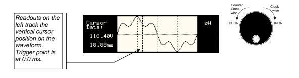
Figure 4-35: Scrolling through acquired waveform data
