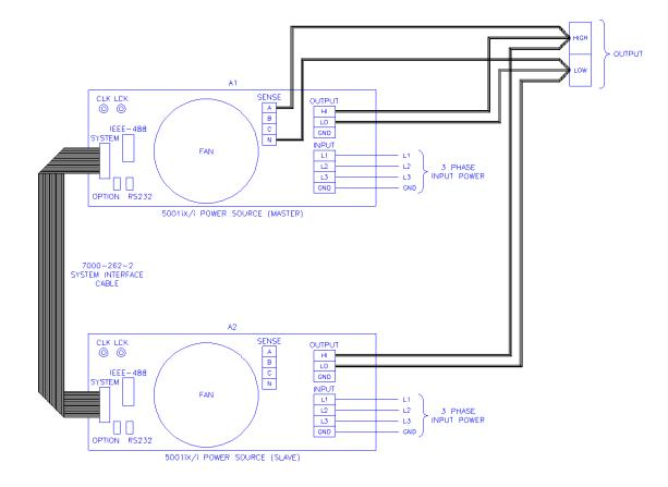
Figure 3-9: Single Phase 10000 VA System (10001iX/i)
