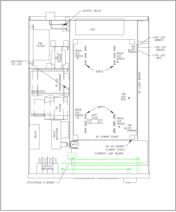
Figure 5-3: 5001i Internal Layout
