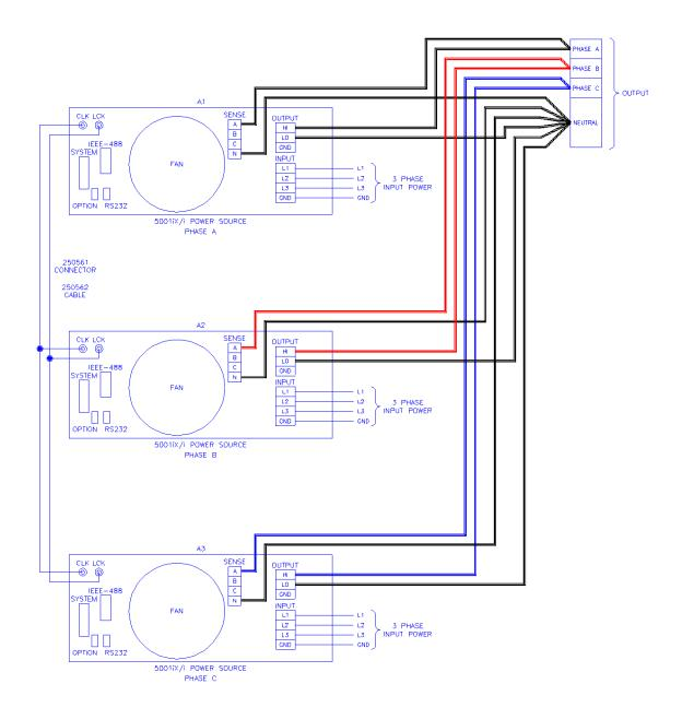
Figure 3-10: Three Phase 15000 VA System (15003iX/i-LK Three Controllers)
