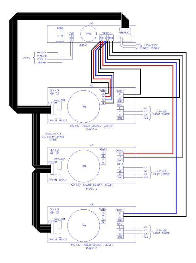
Figure 3-13: Connection With MODE Option
