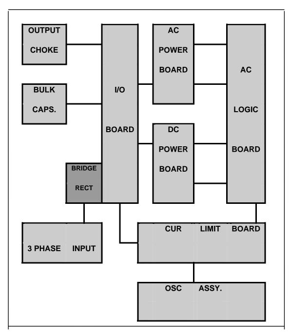
Figure 5-1: AC Power System Block Diagram
