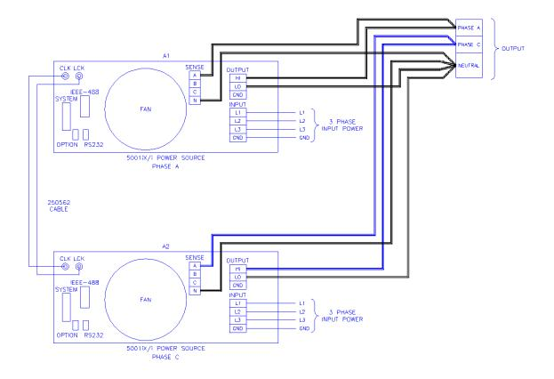
Figure 3-14: Two Phase 10000 VA System (10002i-LK Two Controllers)
