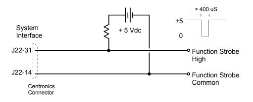
Figure 3-3: Function Strobe Connection.
