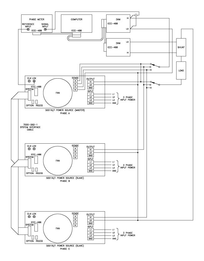
Figure 6-2: Test Equipment Hook-up for Measurement Calibration
