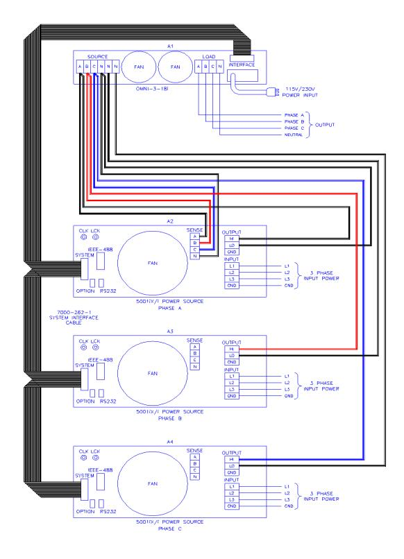
Figure 9-43: Example Connections With OMNI 3-18i
