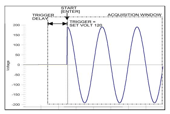
Figure 4-36: SET VOLT trigger source acquisition
